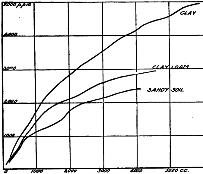
FIG. 55.—Curves showing the absorption of \text{PO}_4 in parts to a million by various soils from a solution of monocalcium phosphate, containing 200 parts to a million of \text{PO}_4 . The volume of the percolate is used as the abscissas.
